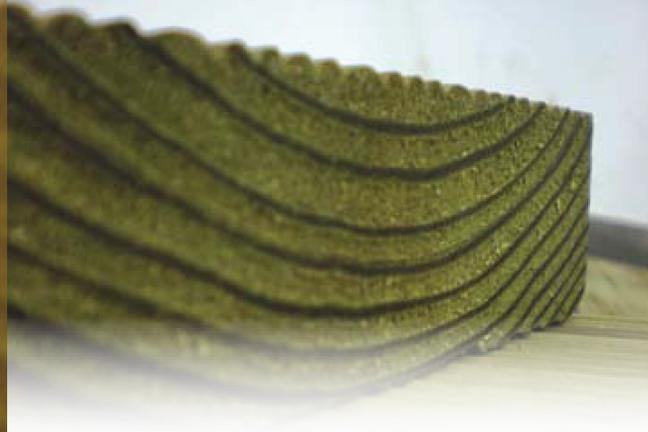
Correctly treated CCA timber that has full sapwood penetration
